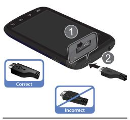
Note: This illustration displays both the correct and incorrect orientation for connecting the charger. If the charger is incorrectly connected, damage to the accessory port will occur therefore voiding the phone's warranty. 4. When charging is finished, first unplug the charger's power plug from the AC wall outlet, then disconnect the charger's connector from the phone.
