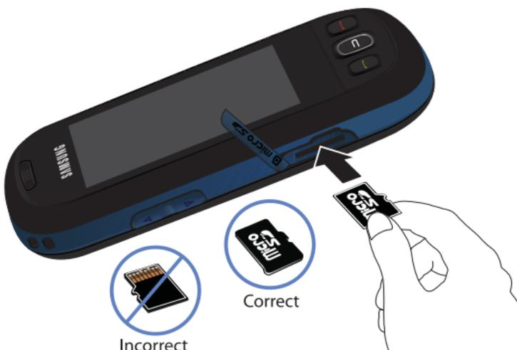
3. Carefully insert the microSD™ card into the opening and firmly push it in until you hear a click, indicating that the card is now securely installed.
