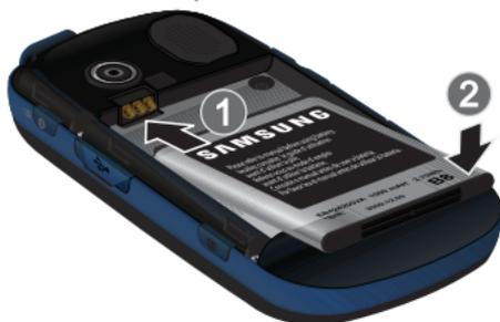
3. Push the top end of the battery down until it snaps into place.
