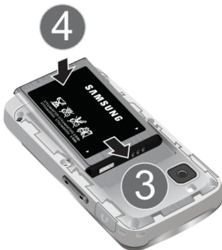
3. To remove the battery, lift the battery up at each end (1) and remove from the phone (2).
